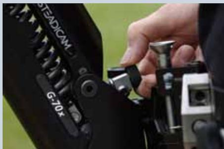
Adjusting the ride: the arm must be angled up at the top of its range. Note: the ride knob is horizontal, the lift knob is vertical.
