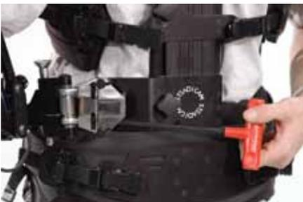
The two side to side screws work independently of one another. Do not tighten the lower screw, but be sure it is all the way in, and then back it out 1/8th of a turn to prevent binding.
