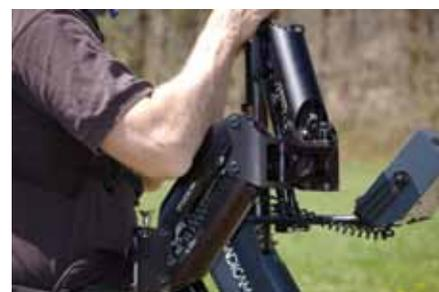
Lift can be altered by forcefully holding the arm segments at the correct angle while adjusting, but be prepared for some exertion! You might be shocked how energetic the springs feel if you are raising or lowering the lift by 30 lbs (14kg)!
