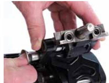
To set your threads, first dial the lower side to side screw all the way in, then adjust the upper screw to your threads - about 2 to 2.5 turns out. Use the same procedure to change back to left side operating.
